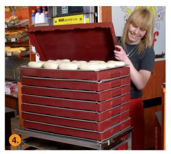
The raw dough comes off the tray residuelessly and falls onto the baking tin in the accurate position.
